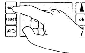
Press the Eco button to switch between Pre-heat (Eco off) and Eco mode. When your Worcester boiler is first switched ON with the optional diverter valve kit, it will be in Pre-heat mode.
