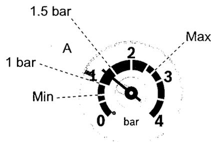
Optimum system pressure when your boiler is cold (area A). If your system pressure is outside area A please refer to section 4 in the user instructions for guidance.
