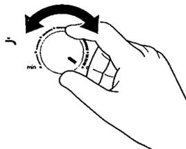
Turn the hot water temperature control knob to the desired level between 40° and 70°C to set the temperature of the hot water within the cylinder. When optional controls are fitted, W100 and FR110, they take over control of the temperature.
