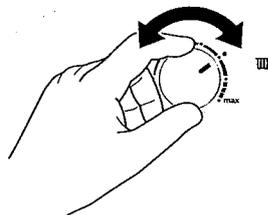
Turn the central heating temperature control knob to the desired comfort level. The "e" point provides guidance for the maximum temperature setting for optimum energy efficiency.
