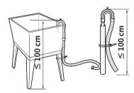
If the drain hose is too long, do not force it back into the appliance. This will cause abnormal noise. • When installing the drain hose to a sink, secure it tightly with string.
