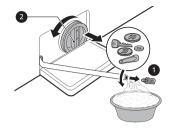
4 After cleaning the drain pump filter, carefully reinsert the filter and screw the drain cap back in clockwise carefully to avoid cross threading and leakage. Reinsert the plug back into the drain tube and place the tube into its holder.
