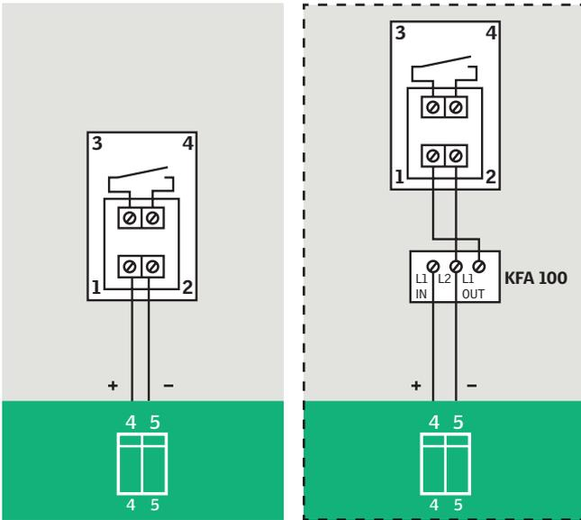
**ENGLISH:** The smoke detector entry can also be used to receive a signal from an external smoke detection system. In that case, a potential free switch and the module shown are required. Fit the module in the external smoke detection system.
