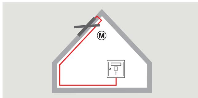
**ENGLISH: Activation via break-glass point:** Break the glass cover and press the red button for at least 1 second. The window opens. (The comfort ventilation function is automatically disengaged).
