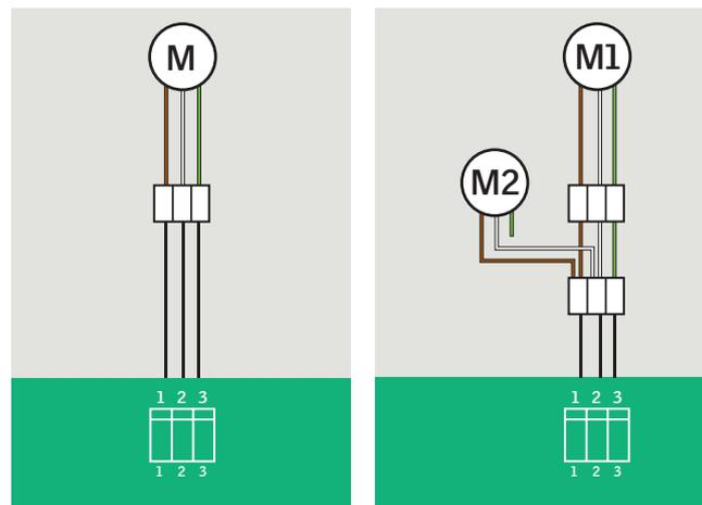
**ENGLISH:** Connect the green cable from the integrated terminal module to the last or only motor. The cables must not be transposed; this would cause malfunction of the integrated terminal module.
