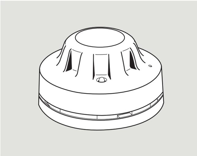
**ENGLISH: Installation:** Smoke detector KFA 100 should always be fitted on the ceiling in accordance with current national legislation. After fitting the base, the smoke detector can be snapped into place. Position dust cover over the smoke detector until it is ready for operation.
