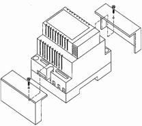
**Important:** Don't cover or obstruct any of the heathsink slots. Wire exactly as the enclosed diagram. Foresee a mains breaker circuit, Don't change fuses with different types ratings.
